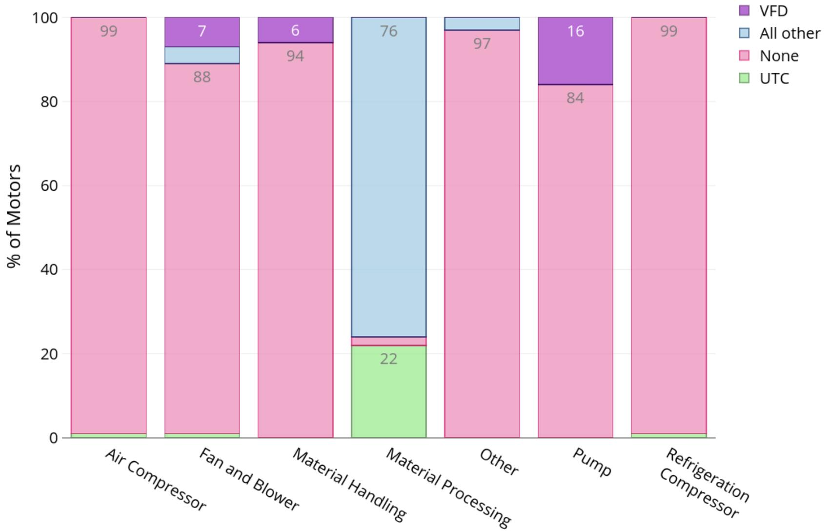
**Figure 71: Penetration rates of VFDs and other control technologies by equipment type in terms of commercial motor system counts. Annotations show the corresponding percent for each segment for shares greater than 5%.**
