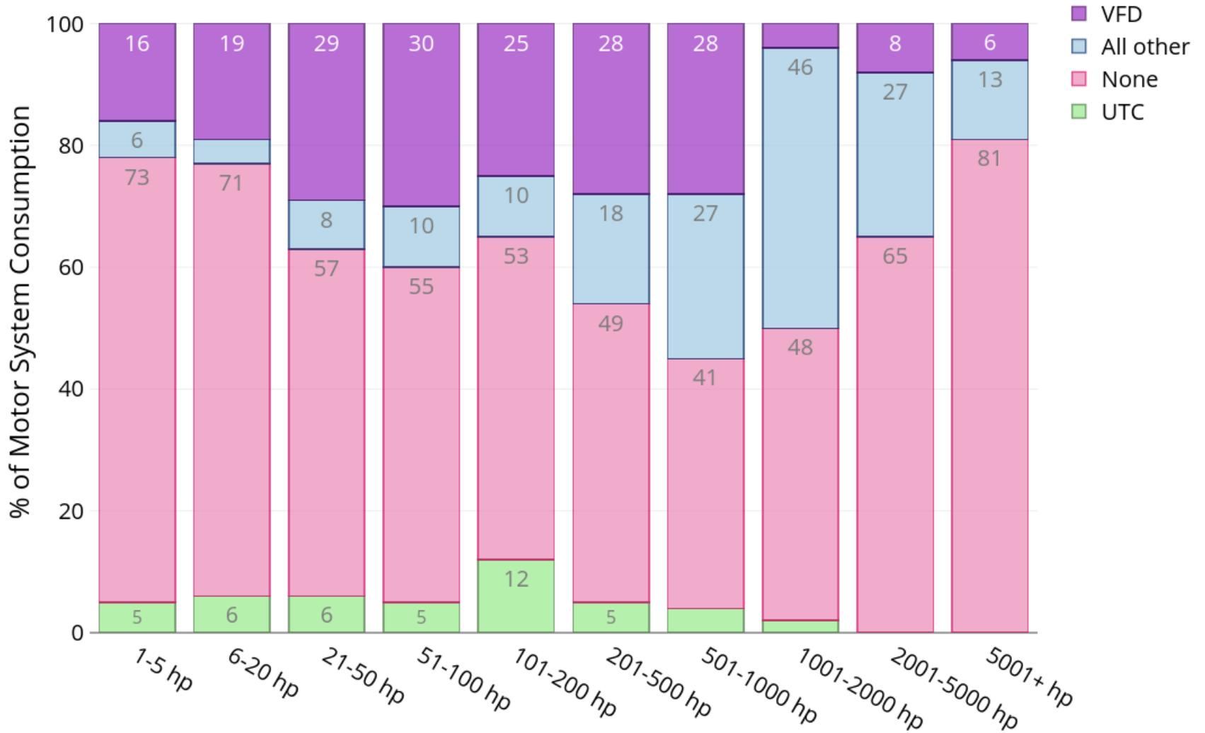
**Figure 61: Penetration rates of VFDs and other control technologies by motor size in terms of percentage of industrial motor system electricity consumption. See Figure 12 for the distribution of connect hp per facility for the industrial subsectors. Annotations show the corresponding percent for each segment for shares greater than 5%.**
