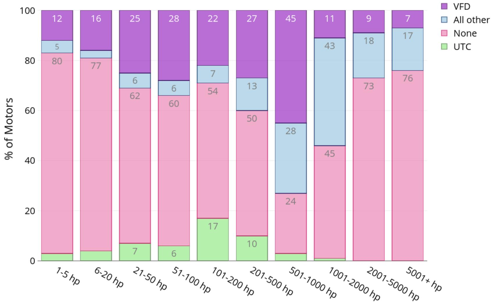
**Figure 62: Penetration rates of VFDs and other control technologies by motor size in terms of percentage of industrial motor system counts. See Figure 12 for the distribution of connect hp per facility for the industrial subsectors. Annotations show the corresponding percent for each segment for shares greater than 5%.**
