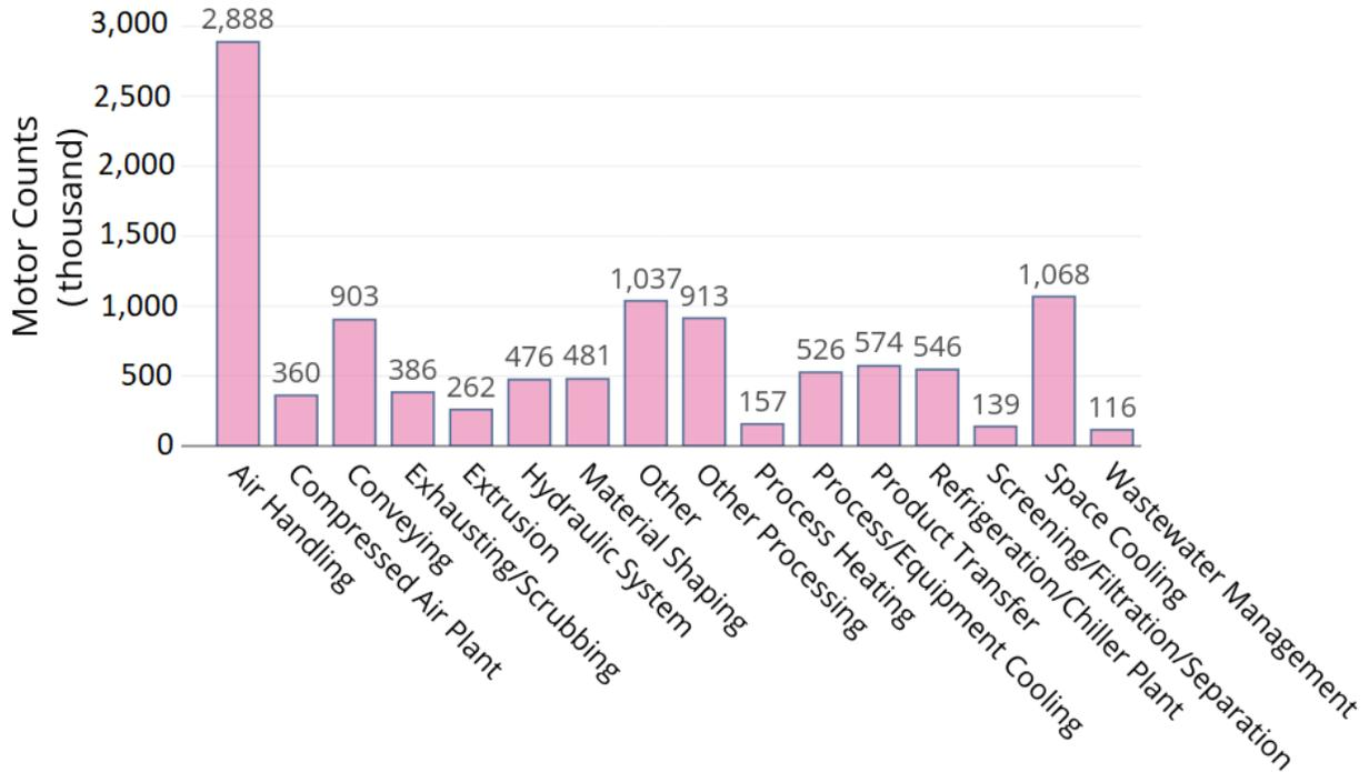
**Figure 28: Industrial motor system counts by process type**
