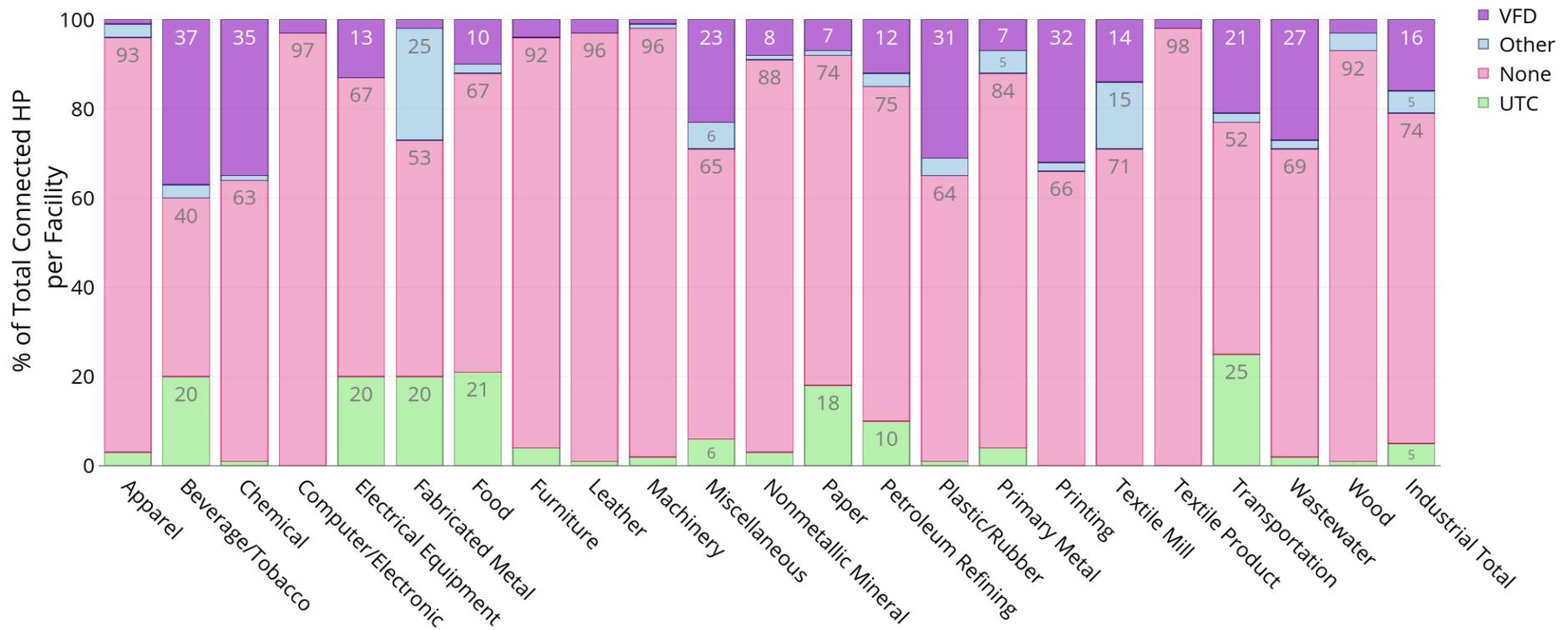
**Figure 59: Penetration rates of VFDs and other load control technologies by industrial subsector. See Figure 12 for the distribution of connect hp per facility for the industrial subsectors. Annotations show the corresponding percent for each segment for shares greater than 5%.**
