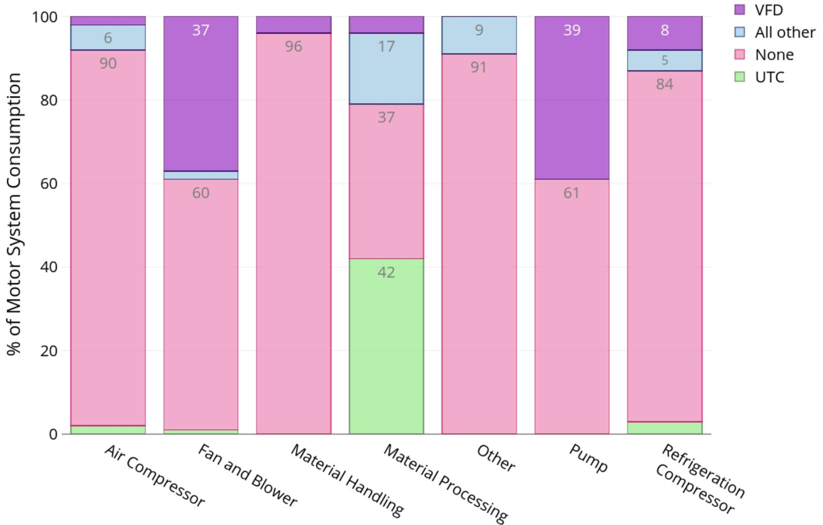
**Figure 70: Penetration rates of VFDs and other control technologies by equipment type in terms of commercial sector motor system electricity consumption. Annotations show the corresponding percent for each segment for shares greater than 5%.**
