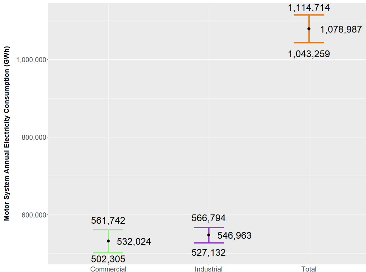
**Figure 6: Estimates of total industrial and commercial motor system annual electricity consumption with 90 percent confidence intervals. Note that the upper and lower bounds of the confidence intervals for the commercial and industrial sectors will not sum to the national level due to the method used for their calculation. The averages do sum.**
