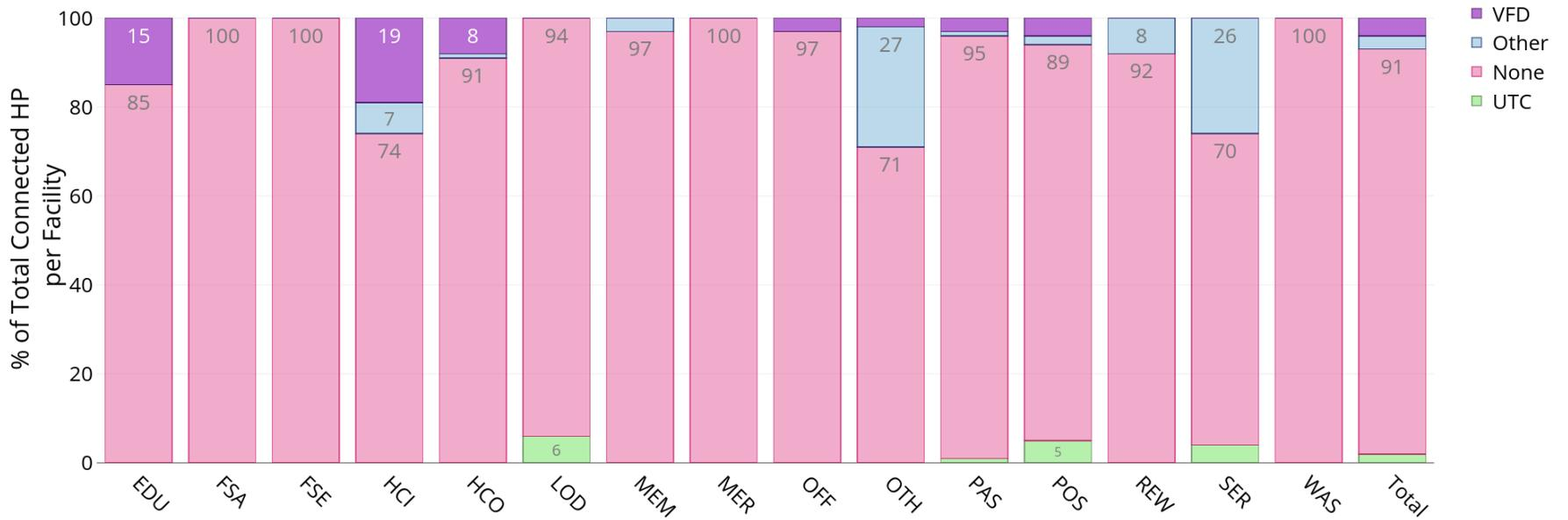
**Figure 66: Penetration rates of VFDs and other load control technologies by commercial subsector. See Figure 17 for the distribution of connect hp per facility for the industrial subsectors. Annotations show the corresponding percent for each segment for shares greater than 5%.**
