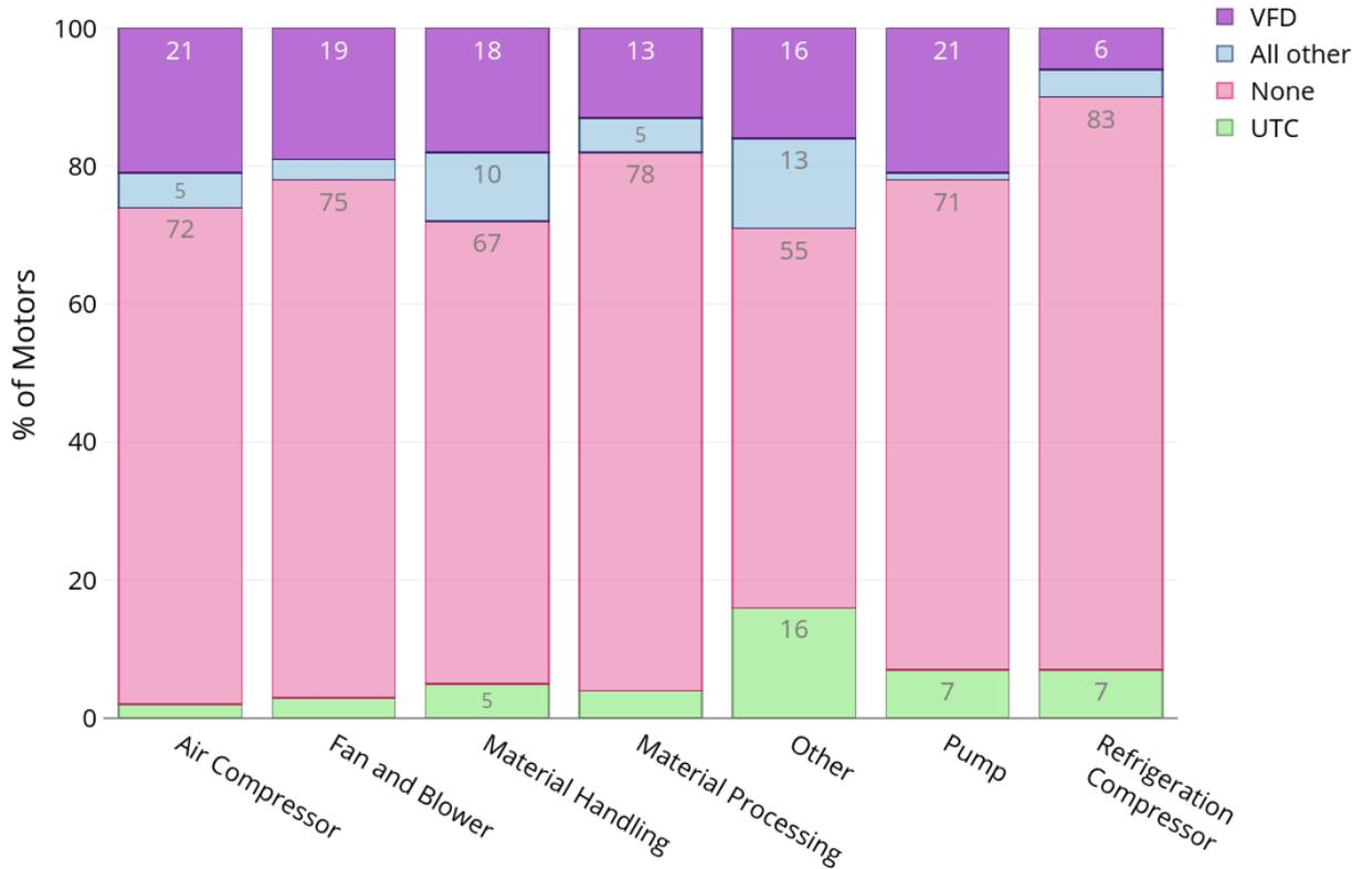
**Figure 64: Penetration rates of VFDs and other control technologies by equipment type in terms of industrial motor system counts. Annotations show the corresponding percent for each segment for shares greater than 5%.**
