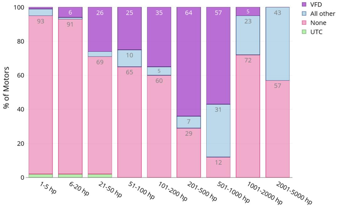
**Figure 69: Penetration rates of VFDs and other control technologies by motor size in terms of percentage of commercial motor system count. Annotations show the corresponding percent for each segment for shares greater than 5%.**
