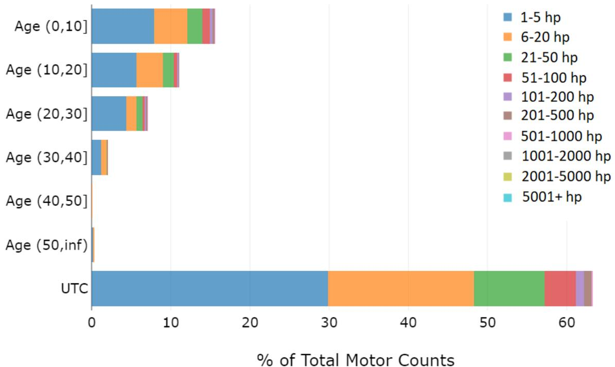
**Figure 51: Age of industrial motor systems broken down by size. Compared to Figure 4, UTC in this figure includes UTC, illegible nameplates, and some nameplates that were legible but the age still could not be determined.**
