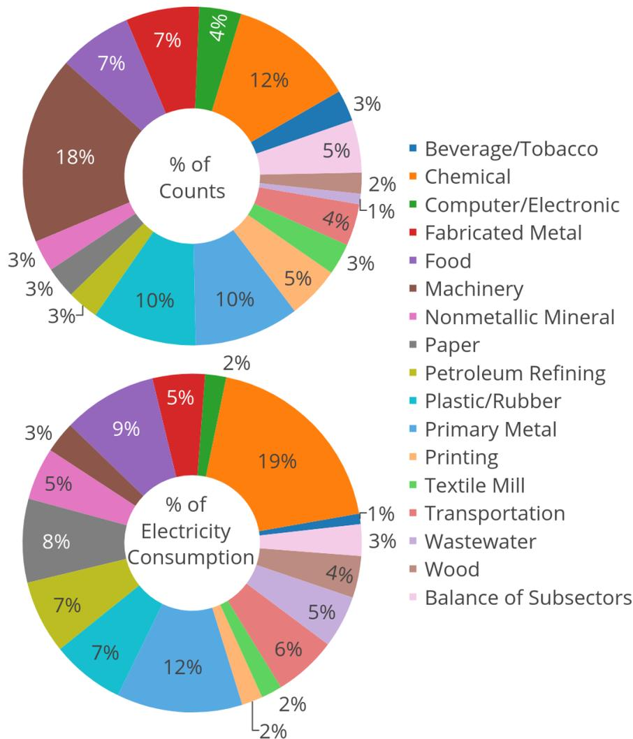
**Figure 11: Share of industrial motor system counts (upper) and electricity consumption (lower) by industrial subsector. The Balance of Subsectors category includes: Apparel, Electrical Equipment, Furniture, Leather, Miscellaneous, and Textile Product.**
