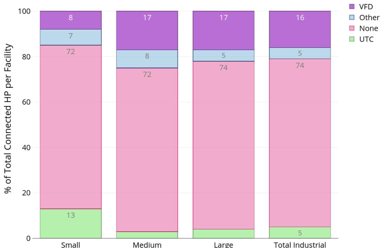
**Figure 60: Penetration rates of VFDs and other load control technologies by industrial facility size. Unlabeled segments are < 5%.**
