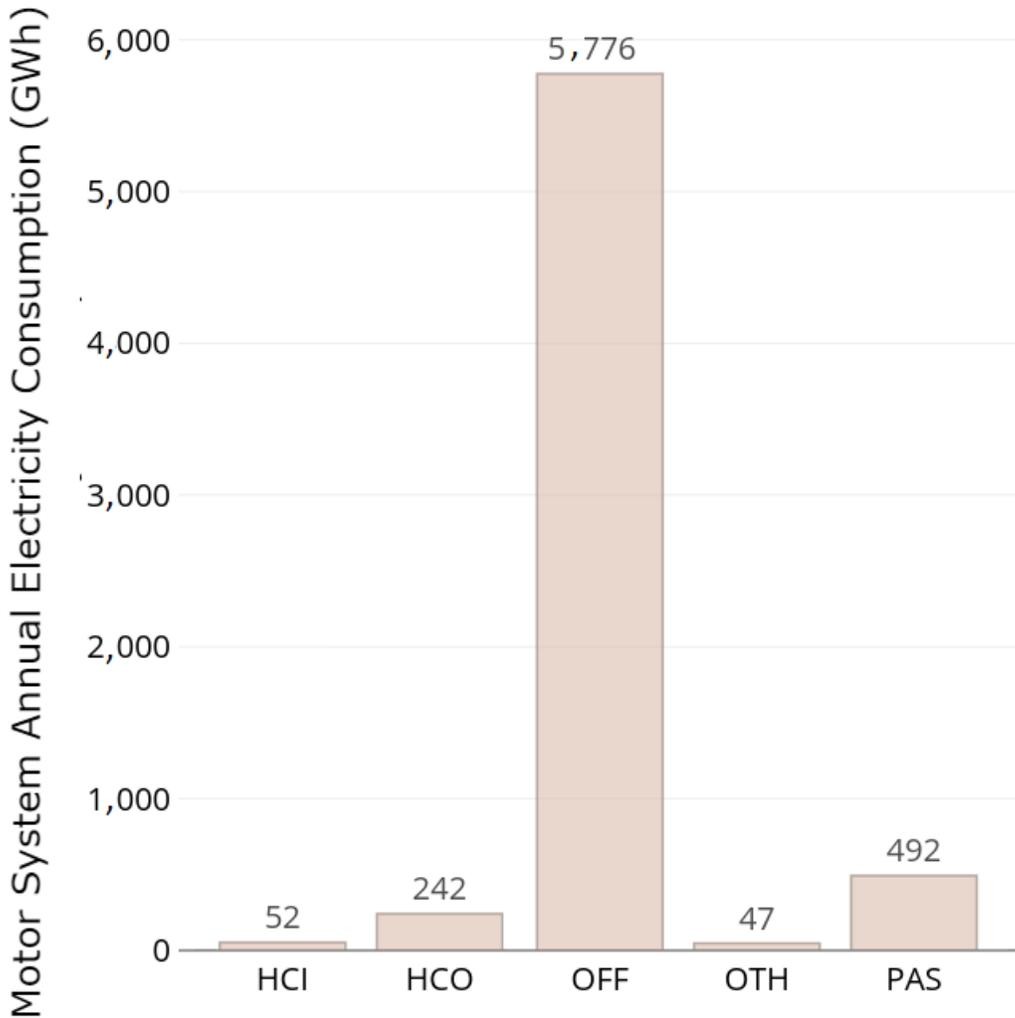
**Figure 47: DC motor system annual electricity consumption by subsector in the commercial sector. Subsectors with no estimated DC motor system electricity consumption have been omitted. These are: EDU, FSA, FSE, LOD, MEM, MER, POS, REW, SER, and WAS.**
