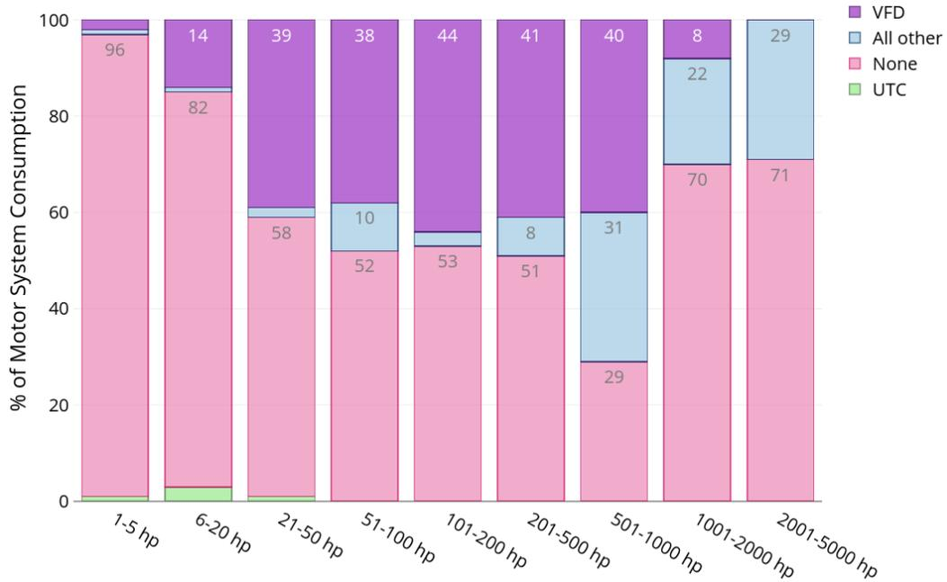
**Figure 68: Penetration rates of VFDs and other control technologies by motor size in terms of percentage of commercial sector motor system electricity consumption. Annotations show the corresponding percent for each segment for shares greater than 5%.**
