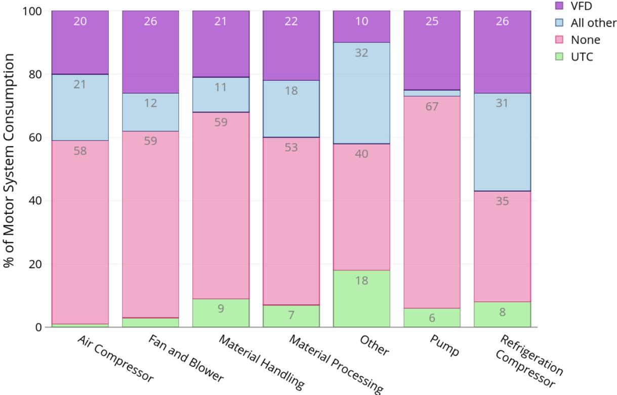
**Figure 63: Penetration rates of VFDs and other control technologies by equipment type in terms of industrial motor system electricity consumption. Annotations show the corresponding percent for each segment for shares greater than 5%.**
