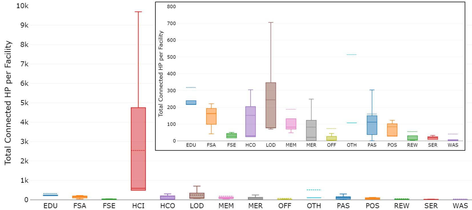
**Figure 17: Distribution of facility total connected hp by commercial subsector. The inset graph rescales the data by removing the Health Care: Inpatient subsector, allowing for the values of other subsectors to be more readily read. Please refer to Figure 5 for guidance on interpreting the box plots.**
